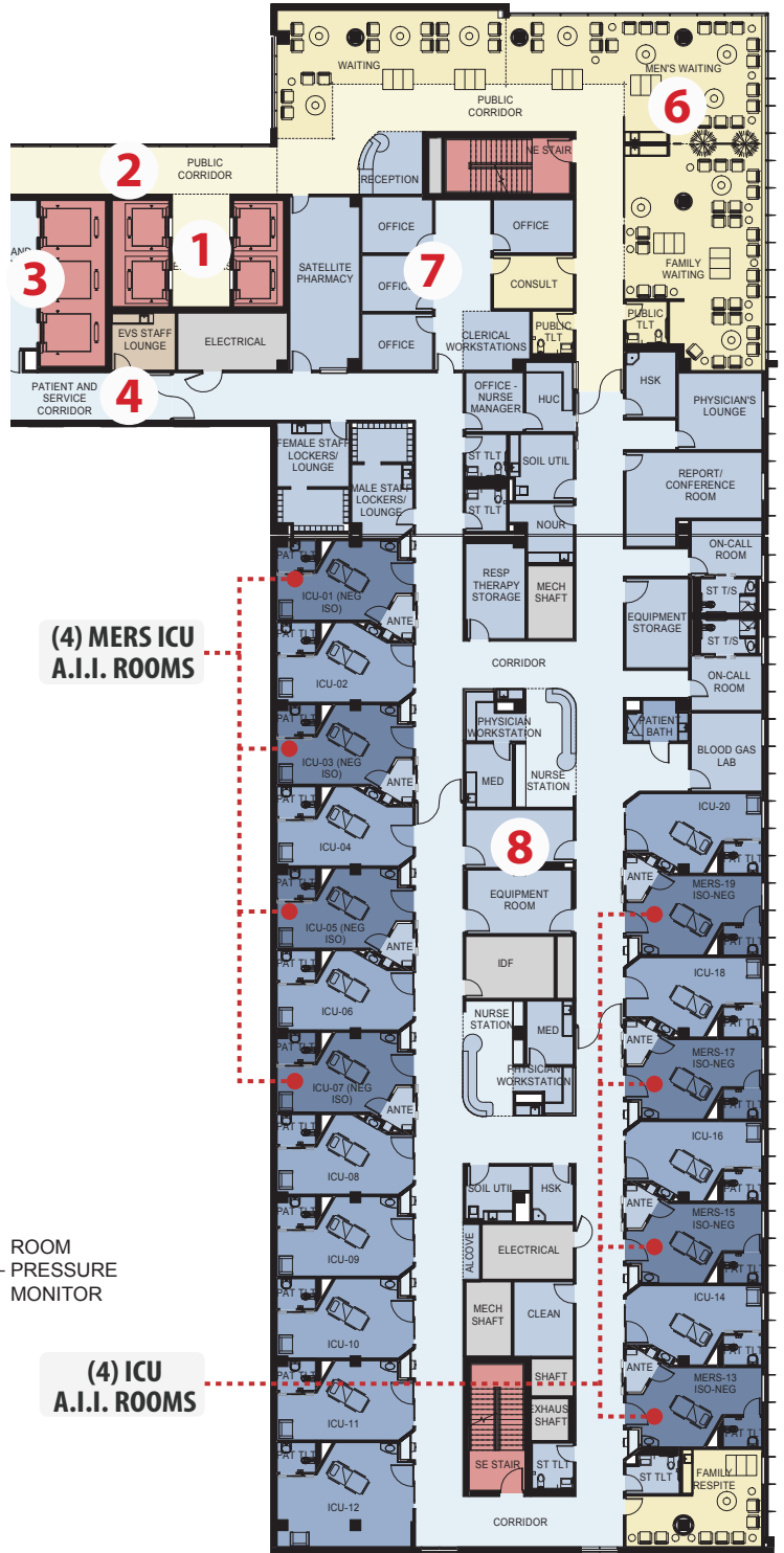
Figure 6: Level Four | 20-Bed Intensive Care Unit
